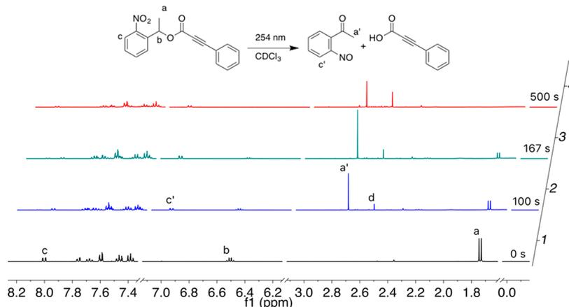
**Figure 2.** <sup>1</sup>H NMR spectra for the photodeprotection of **3b** with a 254 nm UV lamp at a different exposure times. Spectrum 1 was recorded prior to UV irradiation, while spectra 2–4 represent photodeprotection at residence times inside the microchannel of 100, 167, and 500 s, respectively, corresponding to flow rates of 2, 1.2, and 0.4 mL/h, respectively. Furthermore, new peaks a', c', and d emerge, while peaks a–c disappear gradually.
